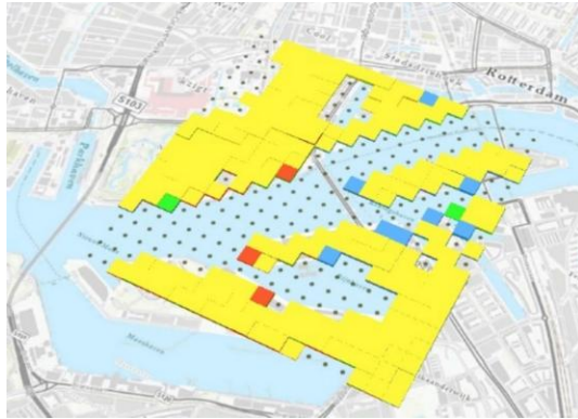
Figure 5 Point dataset representation of the GeoTOP voxel model with selected points rendered as volumetric cells to illustrate voxel origin (left), and corresponding attribute table (right) showing depth-referenced soil types
