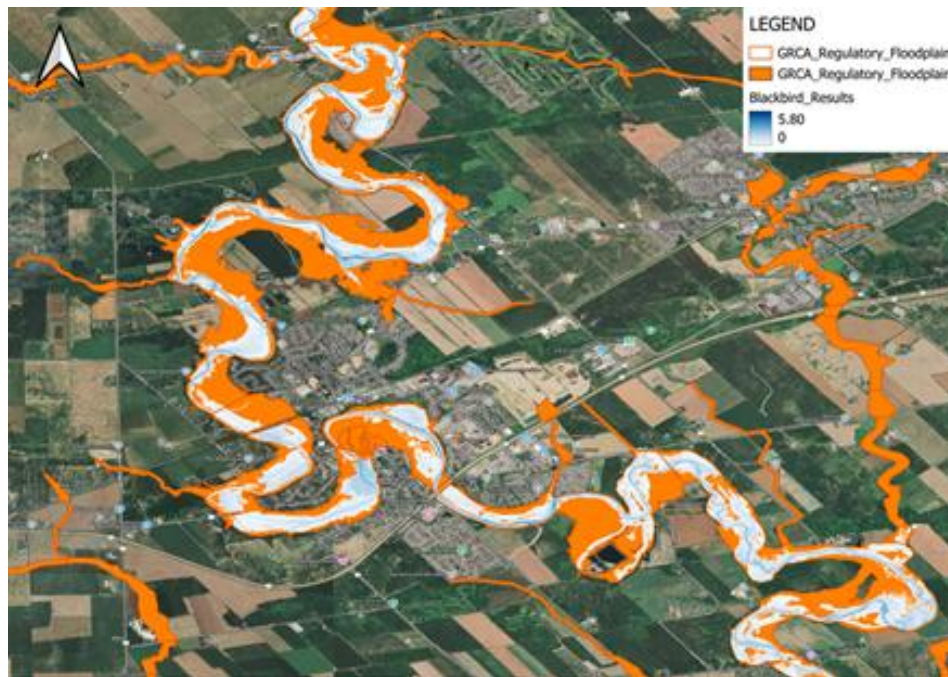
Figure 5 - GRCA regulatory floodplain and Blackbird model output at New Hamburg
